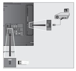
Connect the »USB2 (HDD)« socket of the television and the corresponding socket on the data device (external hard drive, digital camera, card reader or MP3 player) using a USB cable;
